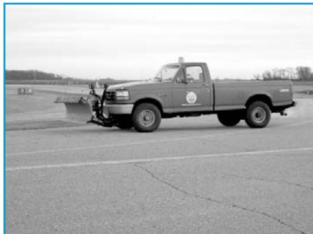
*A maintenance truck with a rotating beacon is used for inspections at the Mankato Airport.*
